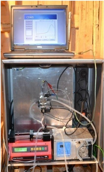
Electrochemical measurements in Screen printed electrodes
